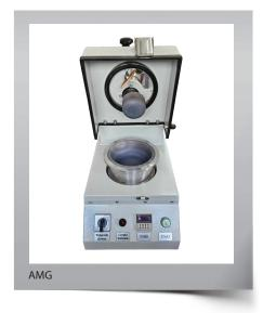
The AMG is designed for grinding of dry and wet hard, medium hard, soft, brittle and temperature sensitive samples. The material is ground under the influence of pressure and friction. The mortar is driven and the pestle is freely rotated and pressed with the adjustable spring. We offer grinding sets made of various materials.
